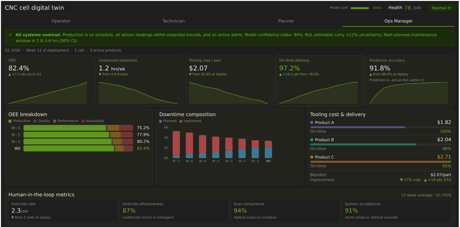
Figure 3.2f. Ops Manager view, Normal state. Five summary metrics with sparkline trends (OEE 82.4%, unplanned downtime 1.2 hrs/wk, tooling cost $2.07/part, on-time delivery 97.2%, prediction accuracy 91.8%). OEE breakdown, downtime composition, per-product cost and delivery, and human-in-the-loop co-adaptation metrics.
