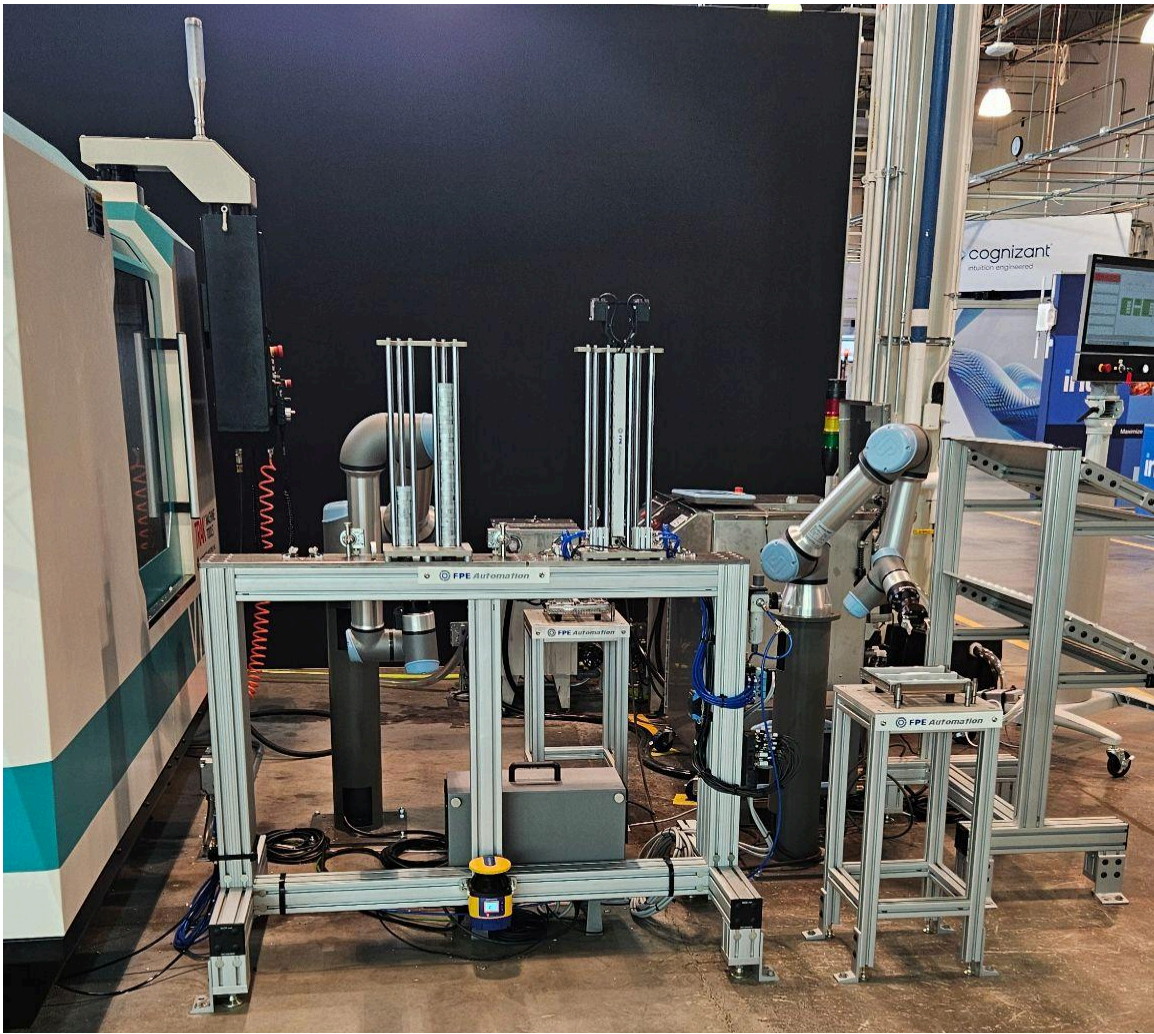
Figure 2.2 Inspiration of the physical setup of the automated manufacturing cell - side view
